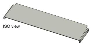
The plate will be installed below the second roller in the S-transition.
